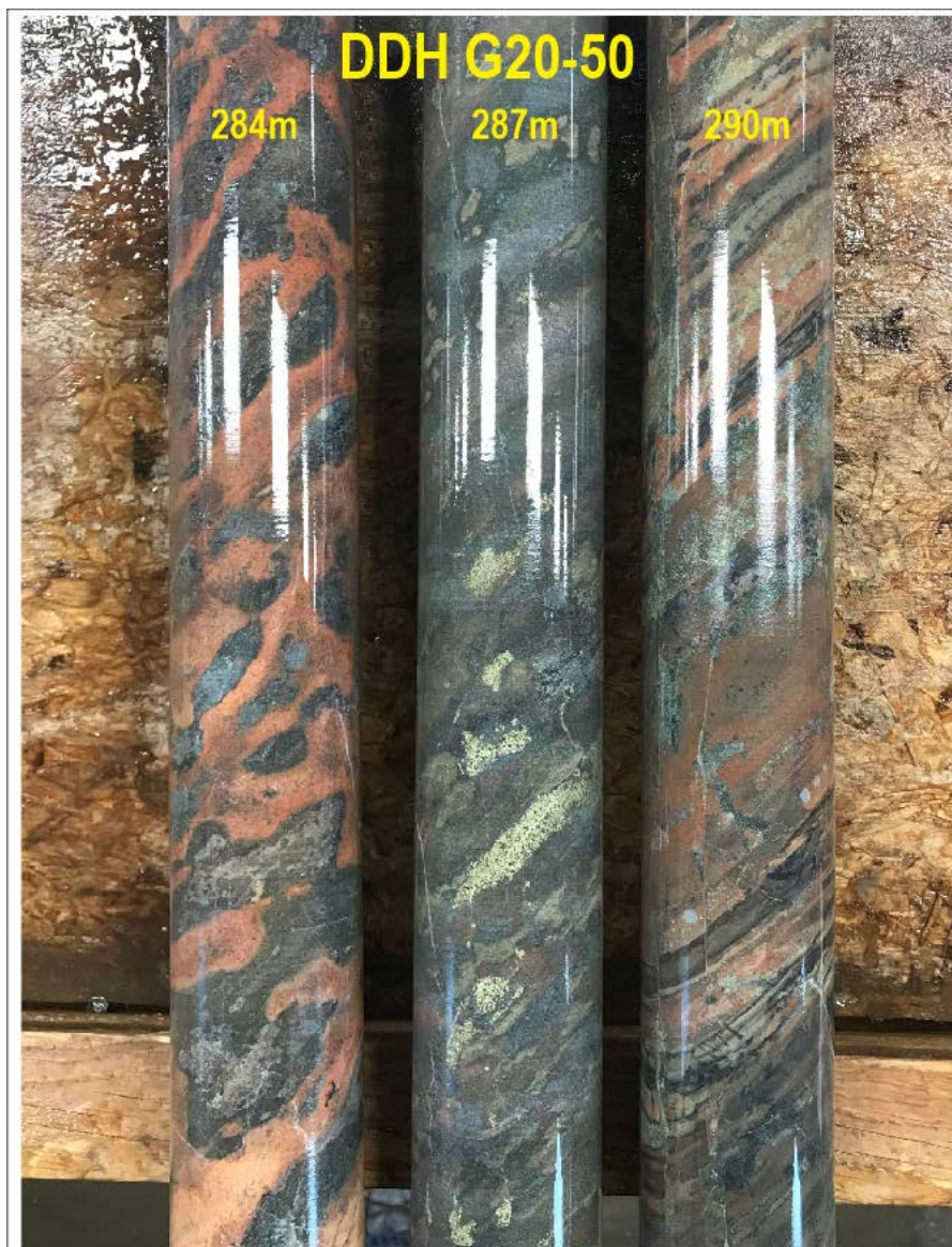
A new zone of CRD (carbonate replacement deposit) mineralization extends south of the Main Zone at G1 and occurs about 50m higher in the stratigraphic sequence. Intense calcsilicate (almandine and grossular garnet-diopside-calcite-epioite-chlorite) of fine grained volcanoclastic sediments obscures original bedding and is associated with magnetite-chalcopyrite-pyrite and tourmaline
