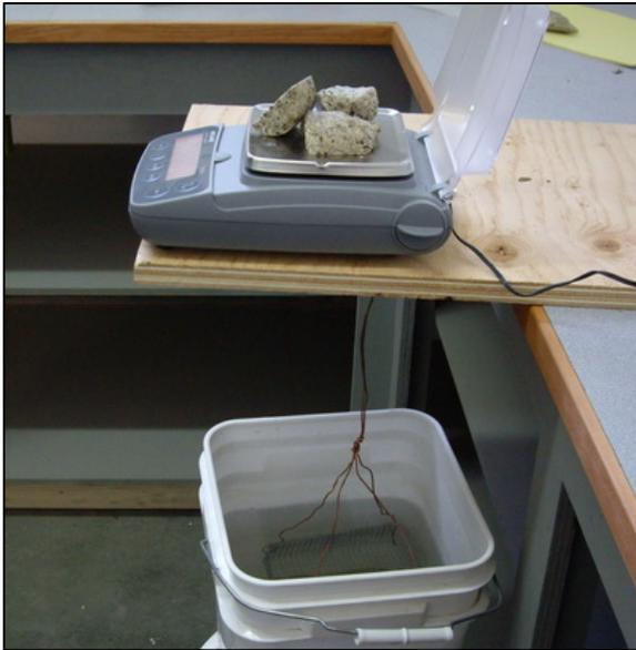
**Figure 10.3: Scale Apparatus used by GWR Staff to Measure the Weight in Air and Weight in Water.**
