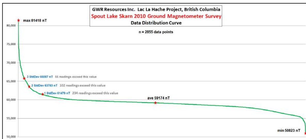
Figure 9-1: Data Distribution Curve for the 2010 Ground Magnetometer Survey over the Spout Zones. Very high magnitudes measured at several sites, where 102 readings exceeded 2 standard deviations, including 55 that exceeded 3 standard deviations. These extreme values were measured directly on outcropping, or very near-surface, massive magnetite with associated copper (gold-silver).
